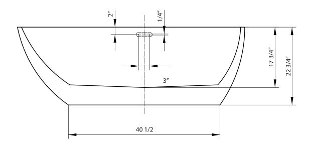
**ATTENTION!** Dimensions may vary by up to 3/8". It is highly recommended to pull all dimensions of actual model for installation and measuring purposes.
